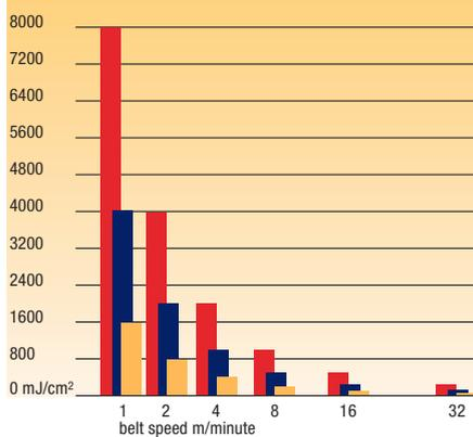
The relation of energy amount and the belt speed is inversely proportional. If speed is doubled efficiency will be half. The higher the initial efficiency the quicker you can cure.
