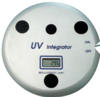
The amount of UV-energy required may vary to a large extent depending on the ink system (measurement values are based on the Kühnast UV-integrator).
