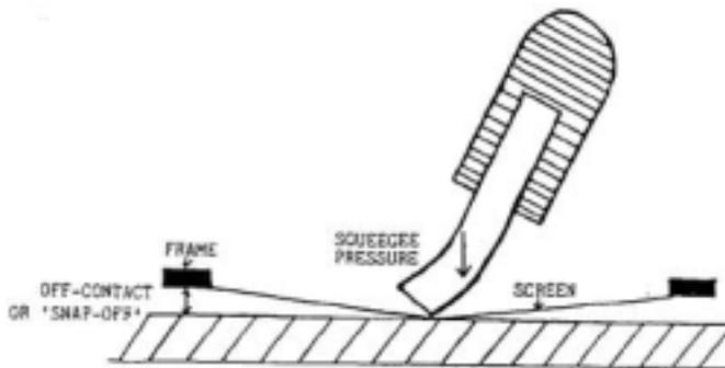
**The squeegee** The squeegee is made of either rubber or polyurethane. The latter material maintains its sharp edge profile on long runs, and is therefore often used in automatic printing presses.
