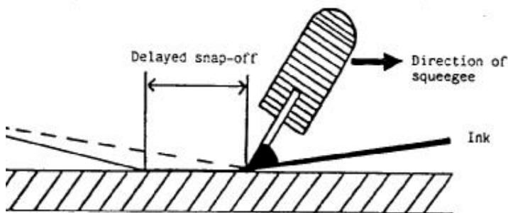
normally done with the aid of mechanical stretching apparatus. Insufficient screen tension can cause delayed screen 'snap off'. With insufficient screen tension a tacky ink will hold the screen fabric to the substrate causing smearing of the print and an uneven deposit of ink.
